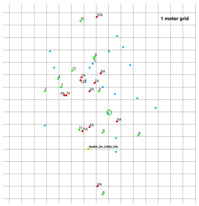
Garmin eTrex 20 in a fixed location indicated by green circle with cross-hair, whose position had been determined with iG3s dual-freq GPS+GLONASS, 350 minute observation time, post-processed by CSRS-PPP with reported 95% probability error ellipse dimensions of 2.4 cm x 1.2 cm.
